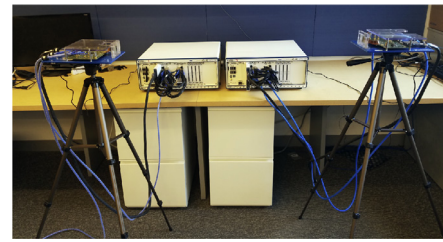
Fig. 1. Two X60 nodes, each attached to a SiBeam phased array module.
