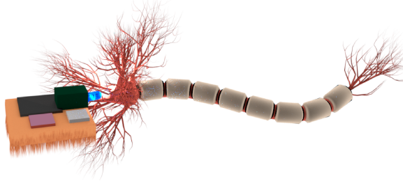
Fig. 2. Illustration of an wi-opt neural dust that interfaces to an engineered neuron that is sensitive to light at a specific wavelength.
