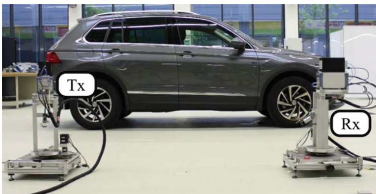
Fig. 15.2 Measuring the vehicle side reflection for the multipath interference modeling at THz frequencies
