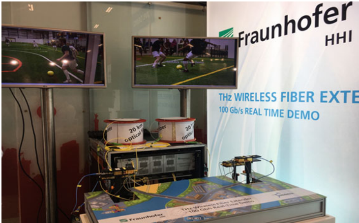
Fig. 35.3 Photograph of the implemented lab demonstrator corresponding to the schematic of Fig. 35.2
