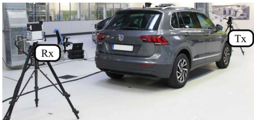
Fig. 15.1 Measuring vehicle-body penetration loss at sub-THz frequencies
