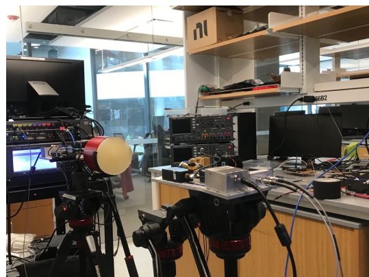
Fig. 5: Experimental Testbed in which the Axicon is mounted directly atop the horn-lens antenna, seen on the left.
