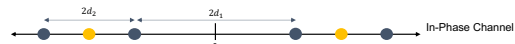
Fig. 6: Constellation diagram for the non-uniform 6-PAM modulation observed by low resolution receiver.
