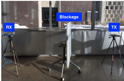
Fig. 8. Experimental setup showing LOS blockage with a wooden table.
