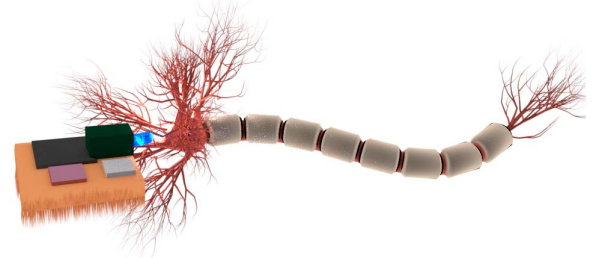
Fig. 4. Illustration of a WiOptND that interfaces to an engineered neuron that is sensitive to light at a specific wavelength.
