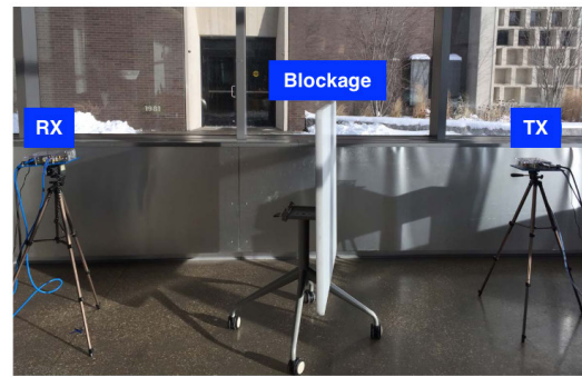
Fig. 10. Experimental setup showing LOS blockage with a wooden table.
