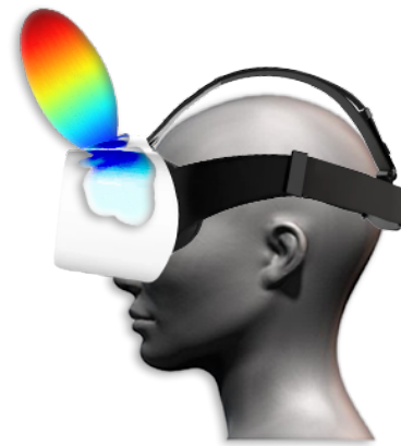
Fig. 1: Electromagnetic radiation emitted from a wireless XR headset with a back lobe hitting the eye cornea.
